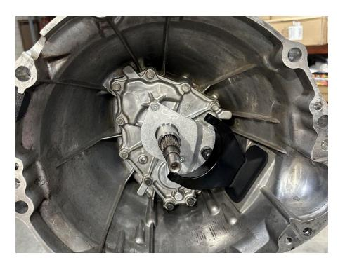
7. Grease the inside of the throw out bearing carrier, you can fully fill the groove with grease. Also add a dab of grease to the bottom of the two 'wings' of the throw out bearing carrier and install the retaining spring for the fork onto the bottom of the carrier.
