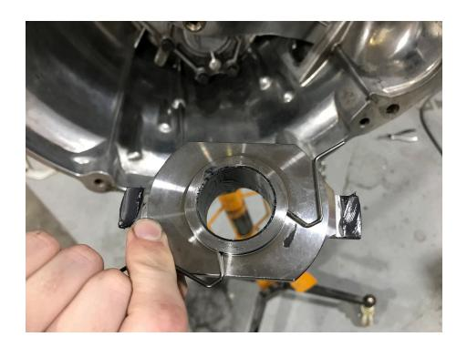
8. Now slide the throw out bearing carrier onto the center guide shaft and seat the fingers of the fork on the wings of the carrier, making sure to slip the ends of the spring into the grooves on the back of the fingers on the fork and clip the two parts together. Then push the assembly all the way back in the transmission and seat the fork with its retaining clip onto the pivot ball. (it should look like this when it's all together on the inside).
