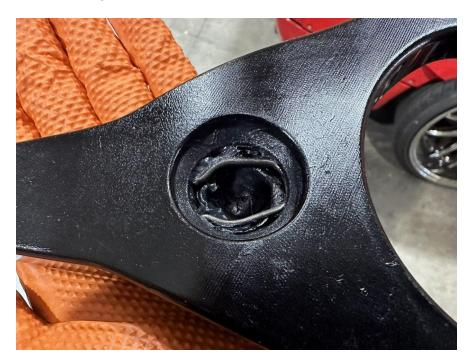
6. Now pop the new boot in place and slide the fork through it and just let it dangle for a second while we prepare the bearing carrier assembly.
