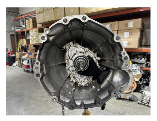
9. Install the braided clutch line, reusing the factory insulative sleeve if possible with some new zipties. Take a second to add a dab of grease to the contact point of the fork adjustment bolt and thread it into the fork if you haven't already, then add its jam nut on the other side. (Torque spec for the union is 11-12 lb-fts)
